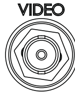
Figure 26-11 View of Video Input BNC Connector from Back of Unit
